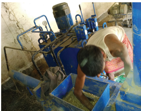
Figure 13. Feed block machine
