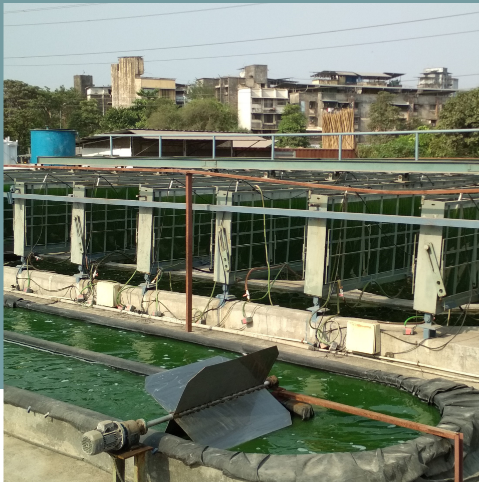
Marine Algal Production System (100,000 L, 220 sq m)
