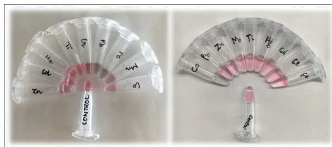
Examples of colour-based sensing of toxic metal ions using capped gold nanoparticles. On the basis of capping of gold nanoparticle, gold nanoparticles displayed colour change in presence of lead/iron (left) and cobalt (right).
